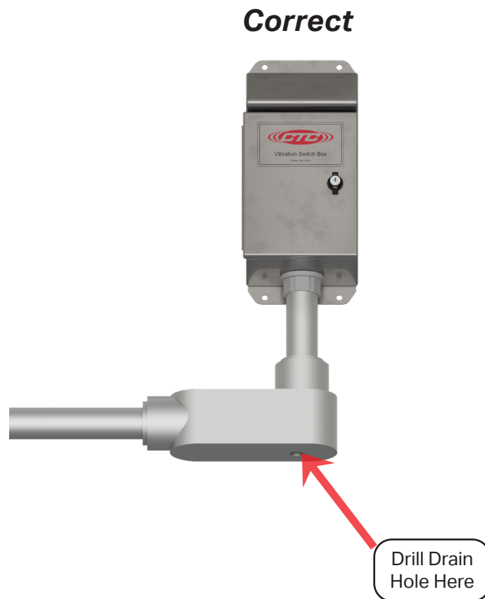
Figure 4. Conduit Entry for Switch Box
