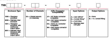
\*No punch outs are provided in the enclosure for cable entry. User may install any fitting required.
